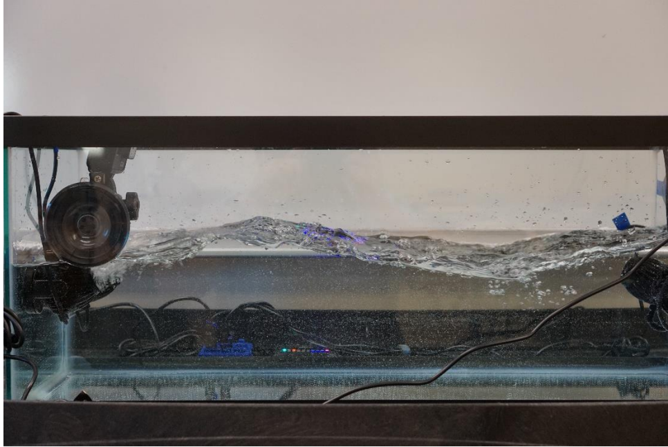
Figure 4. Side view of wave motion after two sets of wave pumps are turned on.
